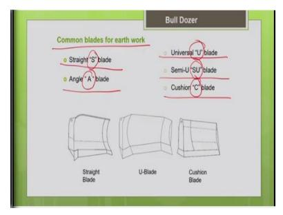
Now let us look into what are all the different types of the blade. These are the common blades which are used for the earthmoving operation, straight blade, angle blade, universal U blade, semi U blade and cushion blade. So, these are the standard notations used S refers to straight blade, A for angled blade, U for universal, SU for semi U and C for cushion blade. So, we are going to discuss all these blades one by one in the upcoming slides.
