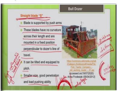
So, first we are going to discuss about this straight blade. Straight blade it is denoted as S, S blade. As the name indicates straight that means your blade is fixed straight perpendicular to the direction of the travel. So, this blade I cannot either angle it to left or right angle it to right, angling is not
