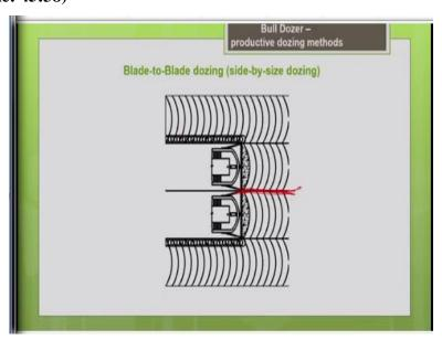
Now let us see another method of productive dozing method to reduce the in spillage. So, here what we are doing is we have to employ 2 bulldozers together and maneuver it in such a way that the blades are coming closer to each other almost touching the blades are brought closer to each
