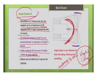
Now let us move on to the next type of blade that is the angle blade. So, these angle blades as I discussed earlier they are connected by C frame. The C frame is connecting the tractor and the blade. So, because of this C frame, it facilitates the angling moment. So, you can see the angle can be turned left or turn right to maximum of say 25 degrees. So, it is mounted on a C frame and can be angled up to a maximum of 25 degree left or right of the perpendicular of the tractor.
