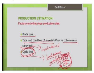
So, obviously your blade type will affect the productivity and the material with the blade is going to push the type of the material, the density of the material all these things will affect the productivity of the bulldozer. How the blade type will affect, we know it already, we have different types of blades straight blade, U blade, angle blade. So, as I told you for hard terrain straight blade will give you high productivity.
