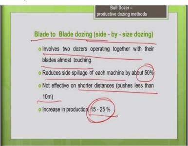
So, this blade to blade dozing it is also called as side by side dozing. Involves 2 dozers operating together with their blades almost touching, it reduces the side spillage between each machine by about 50%. But as I told you like some amount of time is needed for maneuvering, that is why I cannot use it for a very short distance say less than 10 meters, I cannot adopt this method.
