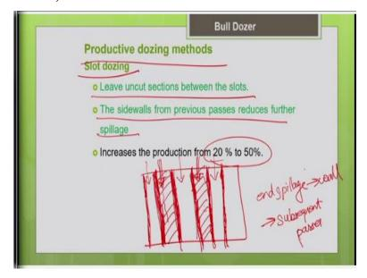
So, one such method is your slot dozing method, slot dozing. So, basically how to carry out this
