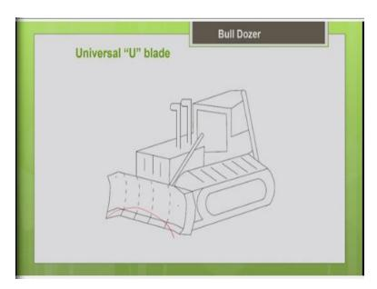
So, this is again a schematic sketch showing the U blade connected to the bulldozer, you can see they are larger in dimension and they have a U curvature. And you can see the wings attached on both the ends.
