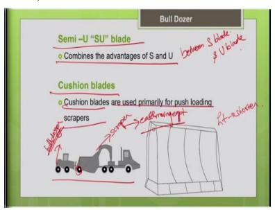
Now let us see what is this SU, semi U blade. It is something between straight blade and U blade, it is between S blade and U blade. That means it is dimensions bigger than the S blade but smaller than the U blade. Similarly cutting ratio is the lesser than the S blade but better than the U blade. So, it is something between the S and U blade. So, accordingly you have to make the choice according to your requirement.
