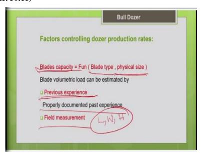
Now let us see how to estimate the blade capacity. The blade, so it is not like a bucket or bowl. So, how much material lies in front of a blade that defines the capacity of the blade. It depends upon your blade type and the dimension of the blade. Obviously as I told you straight blade are smaller
