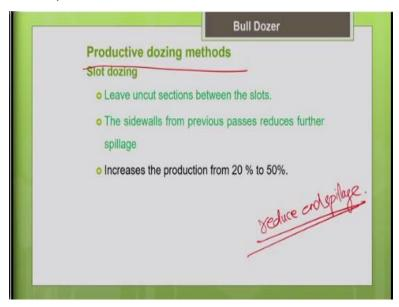
Now let us see what are all the different the dozing methods which are commonly adapted to enhance the productivity of the bulldozer. To enhance the productivity of the bulldozer, I need to reduce the end spillage of the material which is happening at both ends of the blades. How to reducing the end spillage? What are all the dozing methods which can help me to reduce the end spillage?
